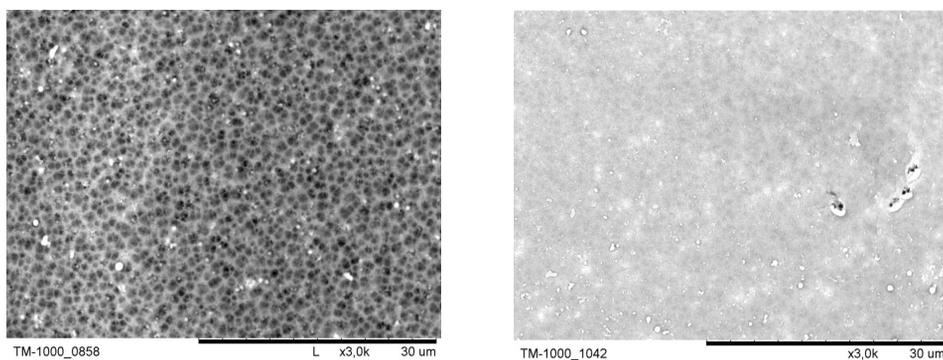
**Fig. 6.** View of the flat membrane with polysulfone cuticle layer designed for cell cultivation. Magnification  $\times 5000$ . The left side of the membrane is unspun and the right side is spun with a gold layer of 30 nm thickness
