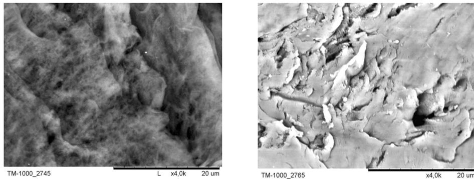
**Fig. 7.** View of the inner polyethersulfone microcapsule surface. Magnification  $\times 4000$ . The left side presents an un-sputtered surface, the right one presents a surface sputtered with a layer of gold of 25 nm thickness
