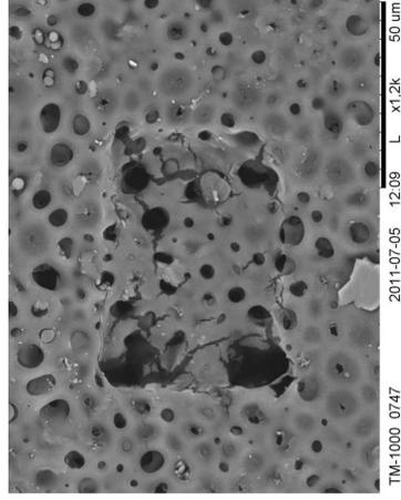
**Fig. 12.** Glicolid/ $\epsilon$ -caprolactone/L-lactyd terpolymer porous membrane sputtered by 15 nm of Au. Left picture magnification  $\times 2500$ , central picture magnification  $\times 2500$ , right picture magnification  $\times 1200$
