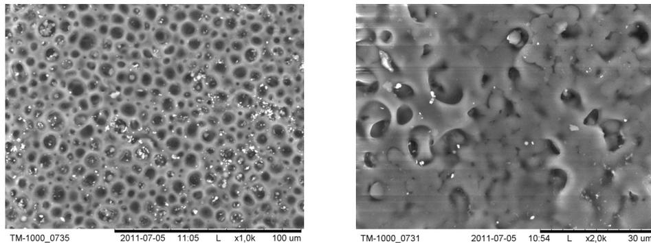
**Fig. 10.** Glicolid/ $\epsilon$ -caprolactone/L-lactyd terpolymere porous, unspattered membrane. Left picture magnification  $\times 1000$ , right picture magnification  $\times 2500$
