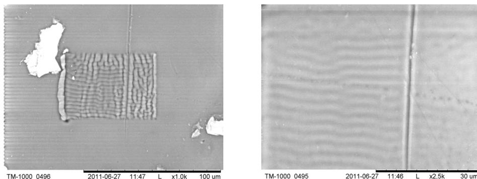
**Fig. 11.** Glicolid/ $\epsilon$ -caprolactone/L-lactyd terpolymere membrane with the close skin layer, melted by the electron beam. Magnification of the left image  $\times 1000$ . Right side: the close-up of the central part of the membrane destroyed by the electron beam (magnification  $\times 2500$ )
