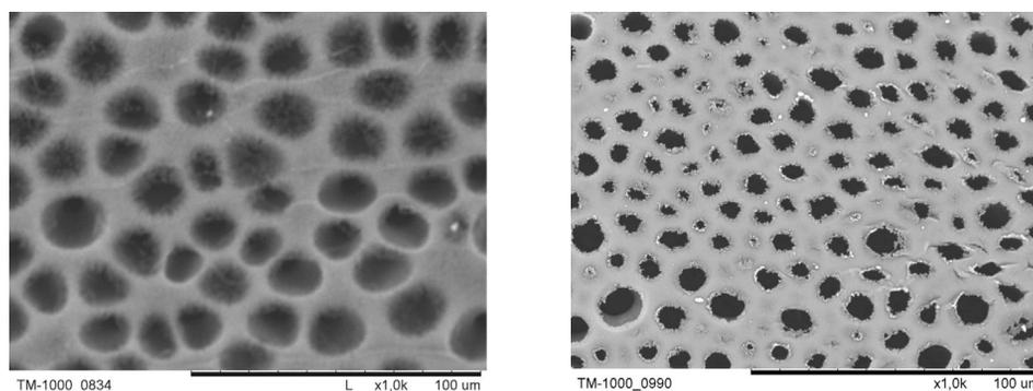
**Fig. 9.** Comparison of the view of the hollow fiber polysulfone membrane of magnification  $\times 1000$ , left – the membrane not covered with a conductor; right – the membrane sputtered by 15 nm Au layer
