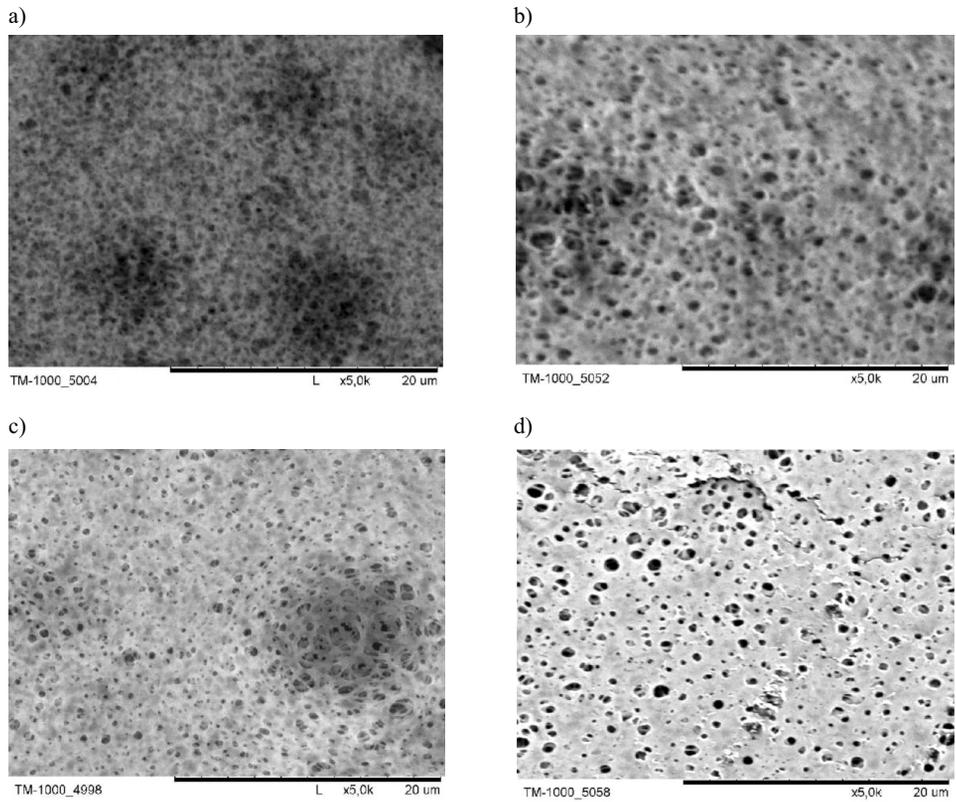
**Fig. 5.** Comparison of the view of the hollow fiber polyethersulfone membrane of magnification  $\times 5000$ . a) the membrane not covered with a conductor; b) the membrane covered with a 6–8 nm layer of Au; c) the membrane covered with a 15–18 nm layer of Au; d) the membrane covered with a 30 nm layer of Au
