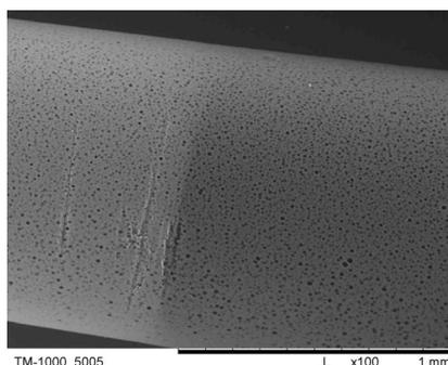
**Fig. 2.** View of the border of sputtering with a gold layer of 5–6 nm thickness. The hollow fiber part sputtered with the conductor is lighter in the SEM picture. Magnification 100×
