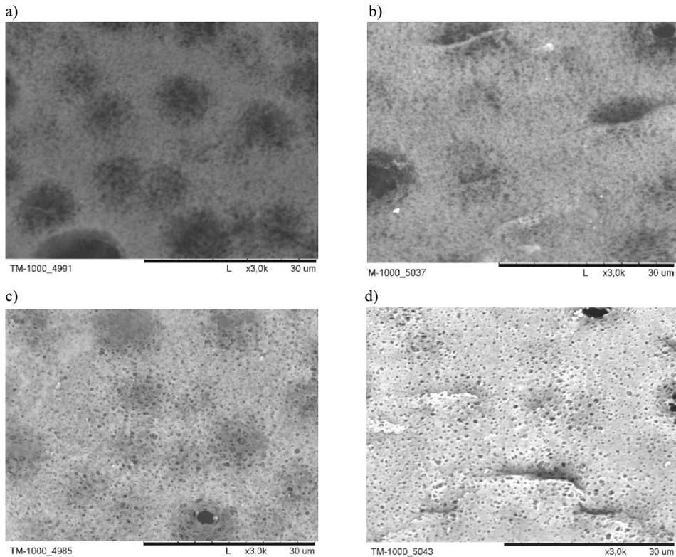
**Fig. 4.** Comparison of the view of the hollow fiber polysulfone membrane of magnification  $\times 3000$ . a) membrane not covered with a conductor; b) membrane covered with a 5–6 nm layer of Au; c) membrane covered with a 12–14 nm layer of Au; d) membrane covered with a 25 nm layer of Au
