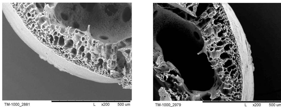
**Fig. 8.** View of the polyethersulfone microcapsule wall ravine. Magnification  $\times 200$ . The left side presents the un-sputtered surface, the right one presents the surface sputtered with a layer of gold of 25 nm thickness
