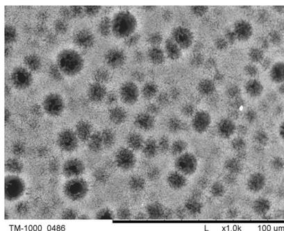
**Fig. 3.** Picture taken without sputtering with a conductor. Magnification  $\times 1000$
