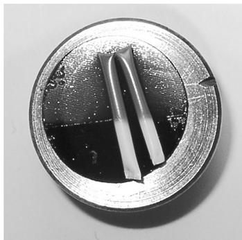
**Fig. 1.** Picture of the supporting table with hollow fiber membranes. Upper half (darker hollow fibers) is sputtered with a layer of gold of 10 nm thickness
