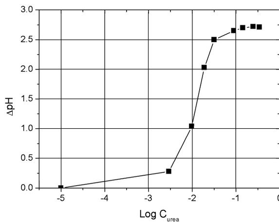
**Fig. 3.** Calibration curve for enzymatic microreactor with urease immobilized onto glass beads ( $C_{\text{urea}}$  – concentration of the urea)
