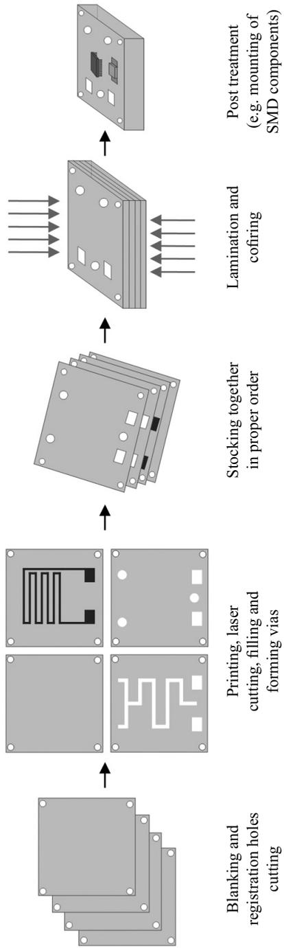
**Fig. 1.** Flow-chart of the LTCC process
