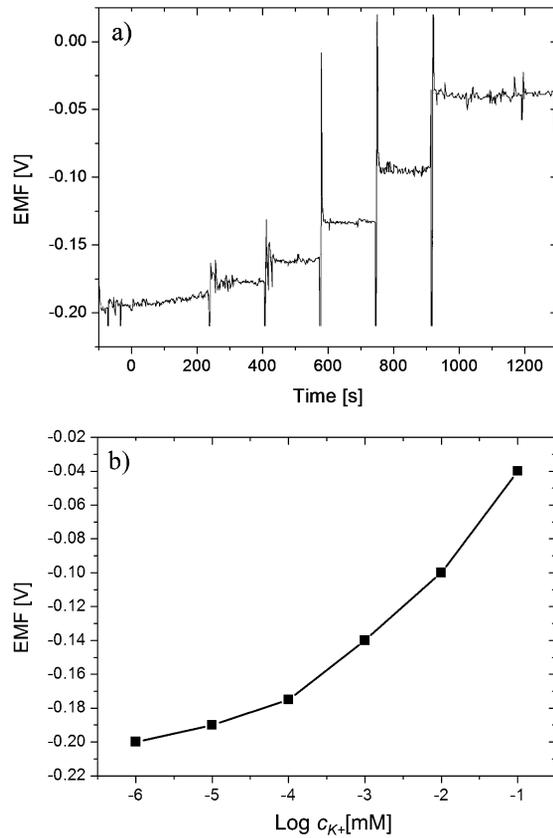
**Fig. 5.** Time responses (a) and the corresponding calibration curve (b) of the LTCC potentiometric sensor ( $C_{K^+}$  - concentration of the potassium ions)
