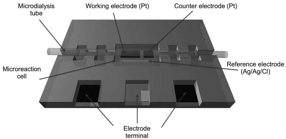
**Fig. 6.** Schematic view of the amperometric glucose sensor
