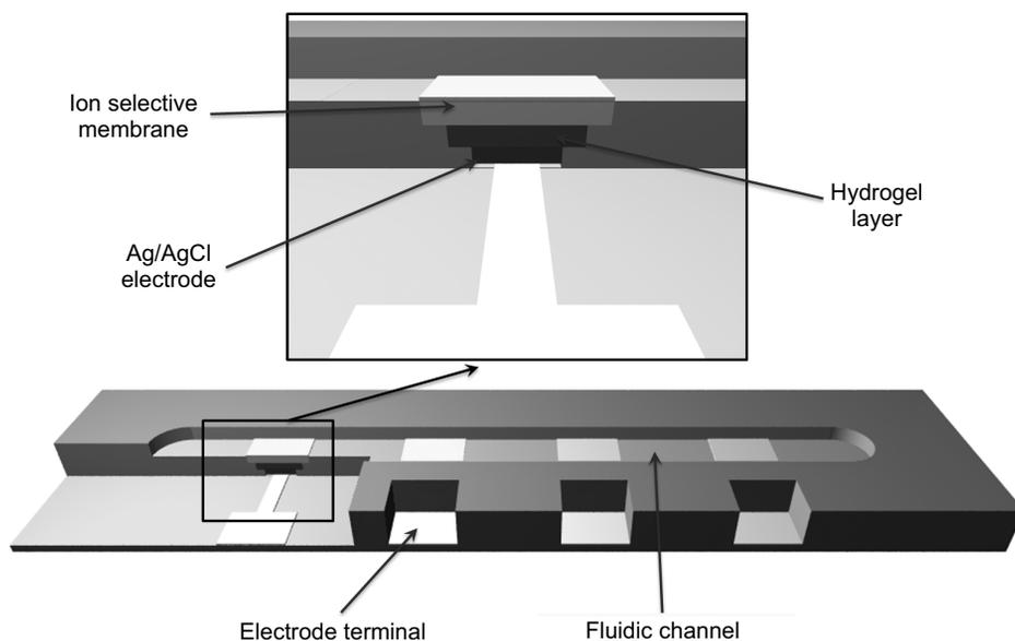
Fig. 4. Schematic view of the LTCC-based potentiometric sensor
