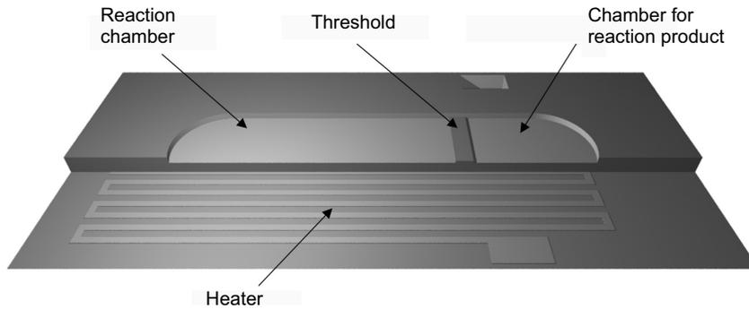
**Fig. 2.** Schematic view of the enzymatic microreactor
