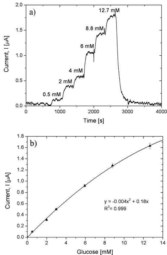
Fig. 7. (a) dynamic response and (b) calibration curve of the LTCC glucose sensor
