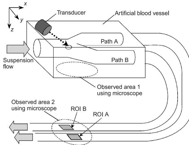
**Fig. 3.** Configuration of the artificial blood vessel, transducer, and two observed areas using microscope to evaluate active path selection of the microcapsules
