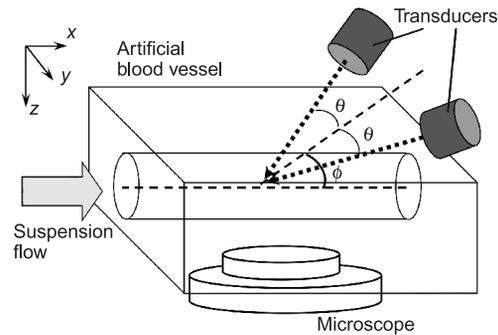
Fig. 7. Schematic view of the experiment to trap the capsules
