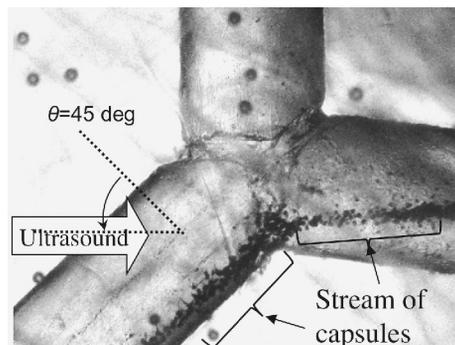
**Fig. 5.** Microscope image of the observed area 1 when injection of the capsule suspension during ultrasound emission
