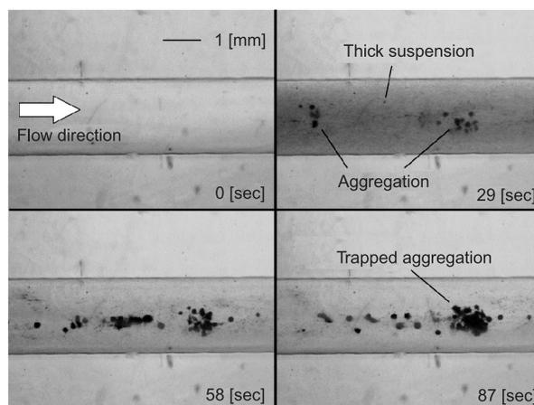
Fig. 8. Time series of the images of the observed area after injection of the suspension with ultrasound emission
