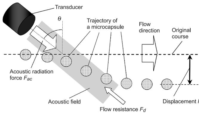
Fig. 2. Trajectory of the microcapsule in flow under ultrasound emission
