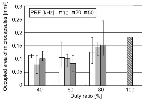
Fig. 10. Average of occupied area of trapped microcapsules versus duty ratio of ultrasound
