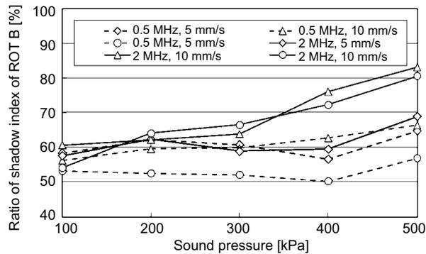
Fig. 9. Ratio in shadow index of ROI B to the summation (ROI A and B) with  $\theta = 45$  degree
