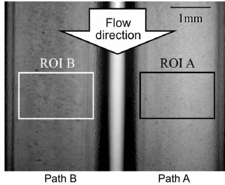
**Fig. 6.** Microscope images of the observed area 2 taken at 300 fps after injection of the capsule suspension with ultrasound emission
