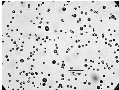
Fig. 1. Microscope image of F-04E microcapsules
