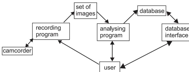
Fig. 2. A schema of the software
