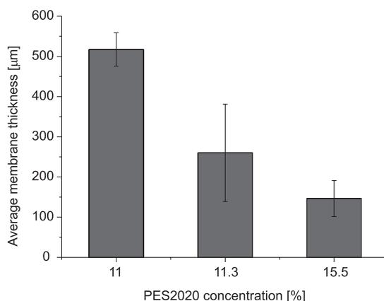
**Fig. 1.** Average membrane thickness in microcapsules produced from membrane-forming solutions of various concentrations of PES2020
