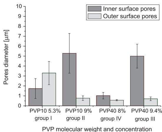
**Fig. 2.** Correlation between PVP molecular weight/concentration and the size of inner surface pores and outer surface pores
