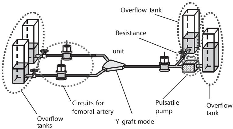
**Fig. 4.** Test circuit for pulsatile flow experiments
