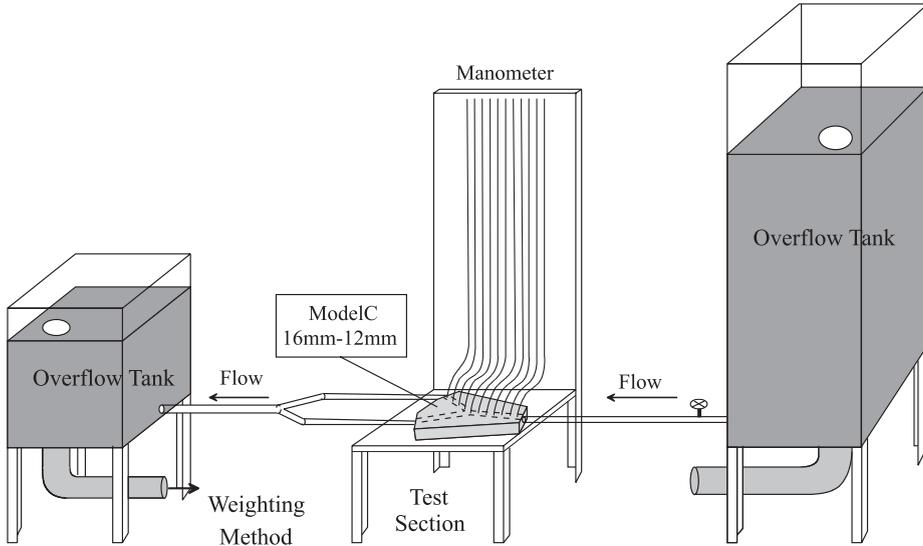
**Fig. 3.** Test circuit used for steady flow study
