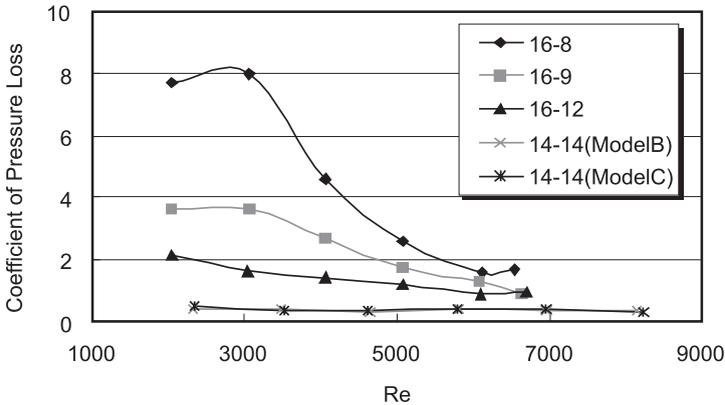
Fig. 6. Coefficients of pressure loss at each Reynolds number
