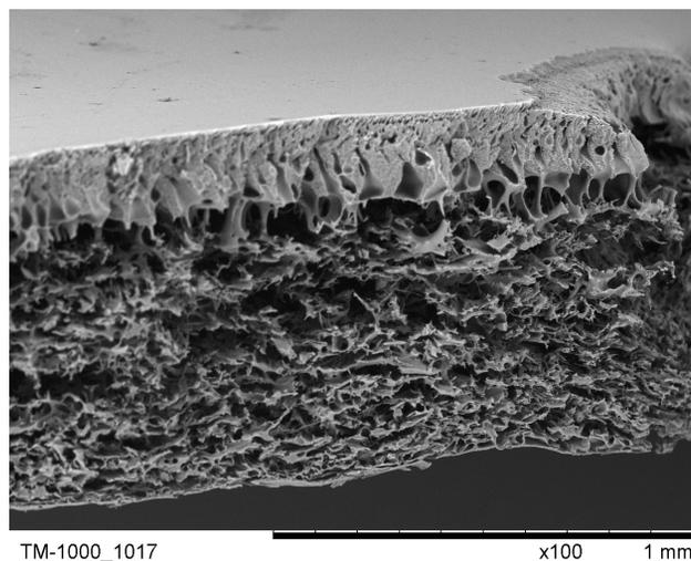
**Fig. 1.** Cross-section through the membrane. Solid skin layer at the top and perforated skin layer at the bottom are visible. The interior of the membrane is filled with a sponge structure. Magnification 100×
