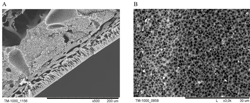
**Fig. 2.** A – Cross-section through the membrane skin layer. The broad-pore membrane skin layer structure is visible. Magnification 500 $\times$ . B – Surface of the skin layer. Magnification 3000 $\times$
