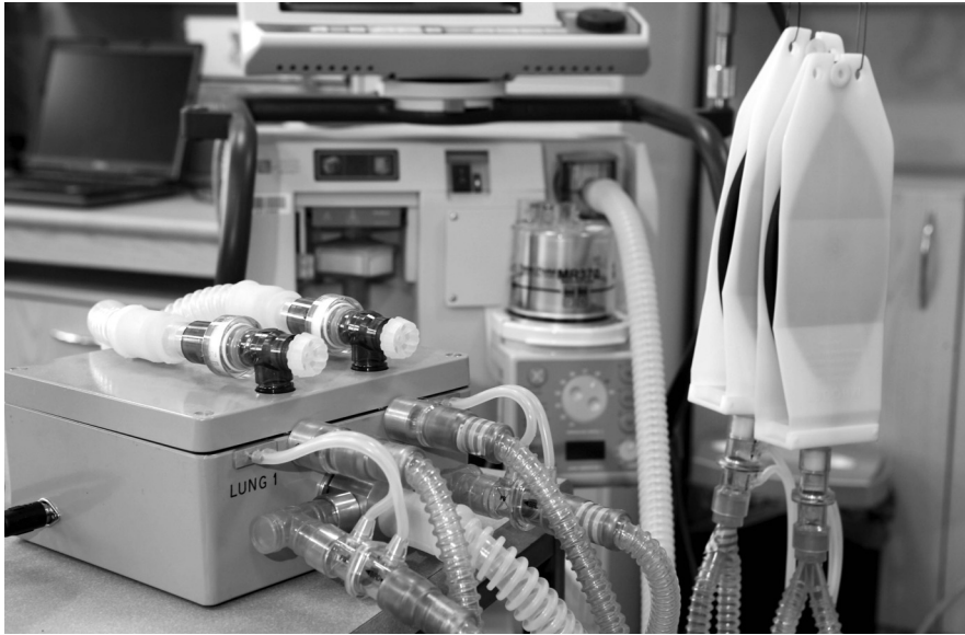
Fig. 1b. Device for independent ventilation connected with respirator and test lungs
