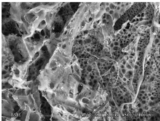
Fig. 1. Membrane of the fourth type – inside the membrane. The picture taken from biological, electron microscope. Enlargement: 500x
